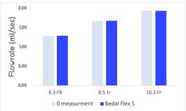
The Bedal Flex S has no measurable impact on the flow.
